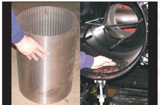
11. Wipe or Brush debris from filter and wipe or brush out housing. Reassemble filter and retainer cap in housing, close cleanout door, check that latches are tight and secure.
