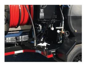
Water system controls mounted near control box and jetter reel for a user-friendly layout.
