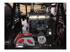
An enclosed engine compartment gives this jetter a clean look with user-friendly access for engine and water pump maintenance.
